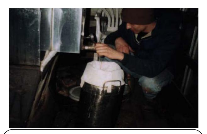
Drawing off the finished syrup is very tricky. It needs to be drawn off at 218 degrees Fahrenheit. If it is cooler than this, the syrup will not be the right consistency. If it is too hot then the syrup will be too thick, and turn to sugar.
