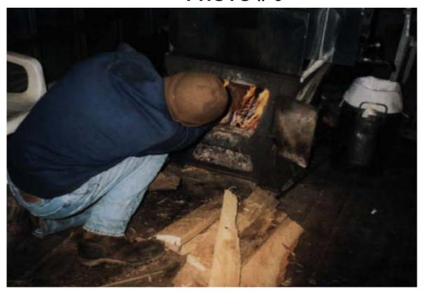
Keeping the fire hot is very important to the efficiency of the evaporator. Since I started making syrup I have improved the boiling efficiency from 15 gallons of sap per hour to 27 gallons of sap an hour. This is about the maximum efficiency my evaporator can handle.
