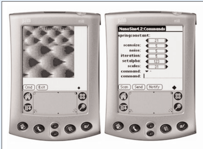
Figure 1: Scanned image of an atomic surface (with a change of scan range) and the parameter screen of the thin client.
