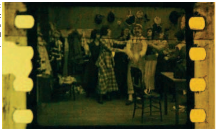
Figure 1: A typical worn-out film-frame with damaged perforation.
