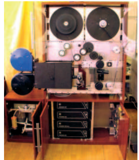
Figure 2: The experimental set-up of the film-saver with scanner and sound correction (in the middle) and film-writer (completely covered on the left-hand side).
