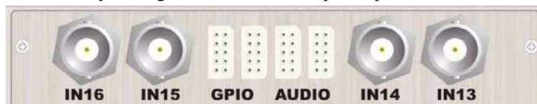
Figure 2-2. VID4 card rear I/O
