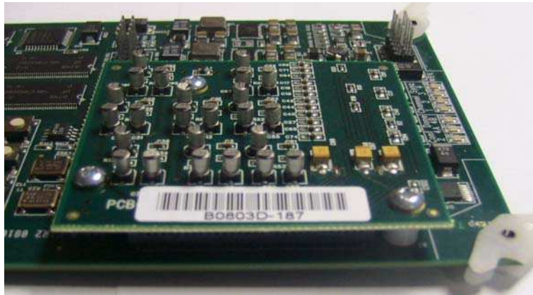
Figure 3-2. Securing an analog audio daughter card in place
