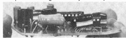
The sophisticated electronics of the Power Chopper consist of a TRIAC, two integrated circuits and several solid-state devices.
