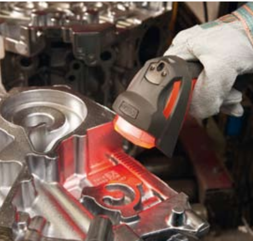
Identification of crankcase with the IT6300 DPM hand-held scanner
