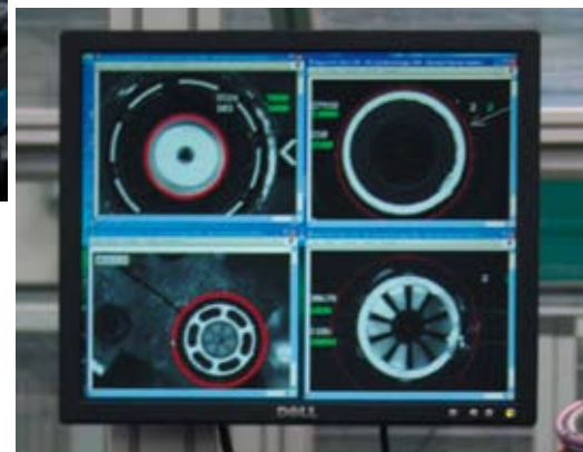
A viewer PC indicates parts assembled incorrectly that were detected by an inspection camera
