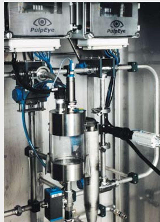
The PulpEye pulp analyzer features the Ranger camera system from SICK IVP that allows calculating ultra-precisely the different components of paper pulp
