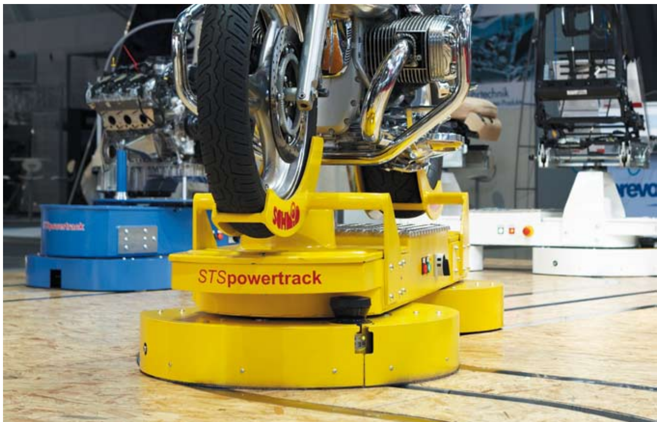
The S300 compact safety laser scanner protects freely moving workbenches
