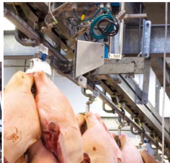
The CLV620 barcode scanner identifies even dirty or partly unreadable barcode labels on the carcasses
