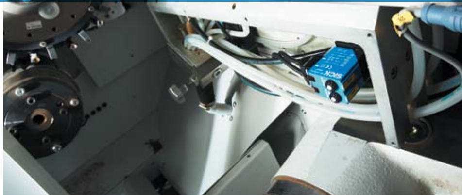
The WLL12 sensor can detect gaps developing between the individual filter rods in the vacuum drum
