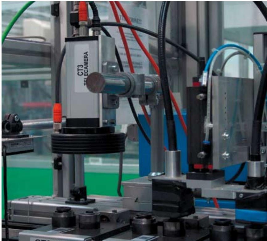
Cameras of the IVC-2D series monitor the assembly process of Lasertyre tire pressure sensors
