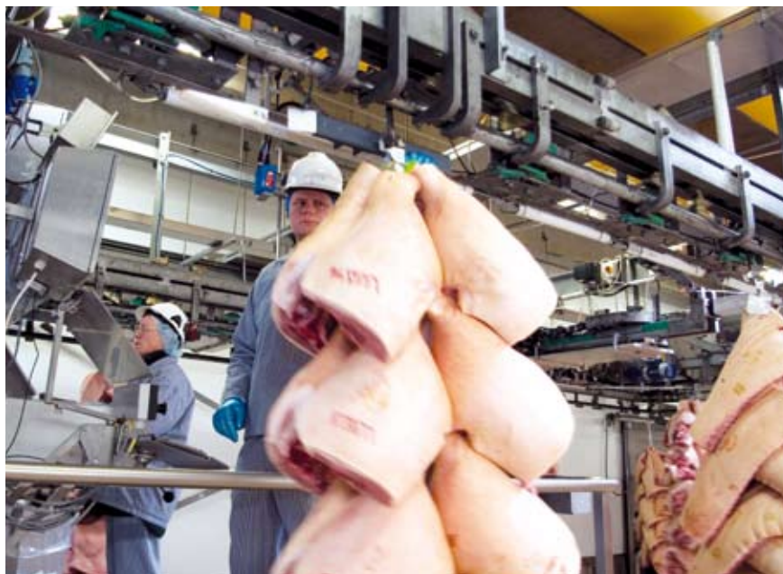
The CLV620 barcode scanner identifies even dirty or partly unreadable barcode labels on the carcasses
