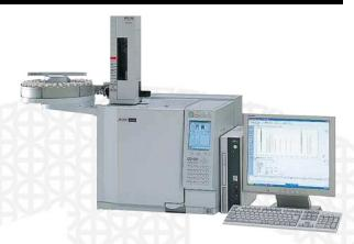
Increase laboratory productivity by automating your analyses with Shimadzu's AOC-20 sample injection system. Proven injection reproducibility is combined with easy operation and high throughput of up to 150 samples.
