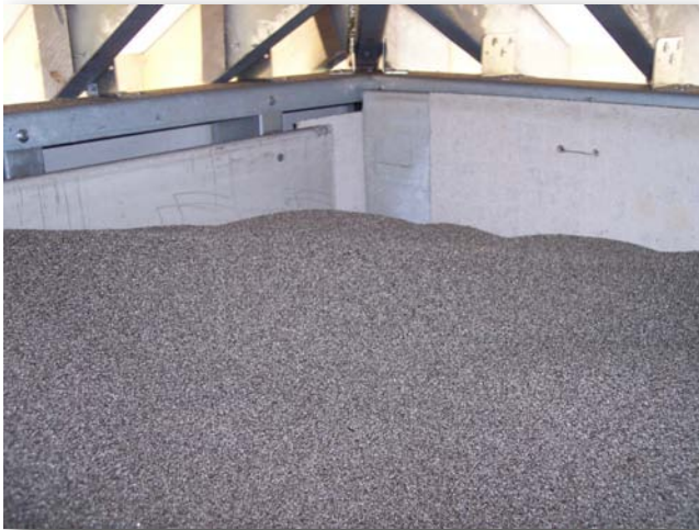
13.4 Loose vermiculite fills a walled enclosure.
