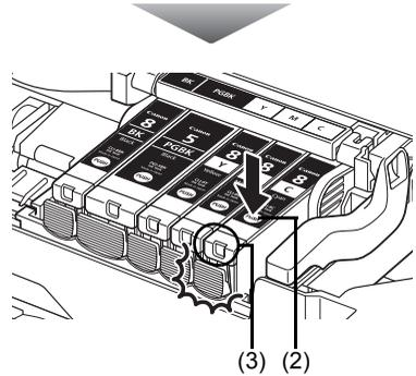
\*1 Make sure the position of the tank matches the label.
