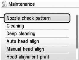
The screenshot shows a vertical menu titled 'Maintenance' with several options: 'Nozzle check pattern', 'Cleaning', 'Deep cleaning', 'Auto head align', 'Manual head align', and 'Head alignment print'. The 'Nozzle check pattern' option is highlighted with a rounded rectangular border. A line labeled '(3)' points to this option.
