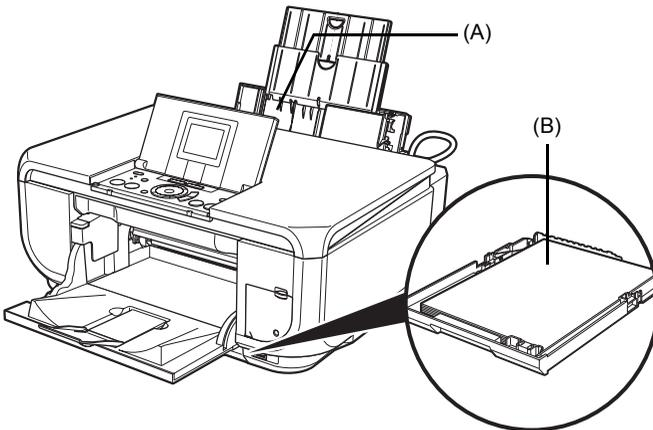
(A) Auto Sheet Feeder: Load paper of various types and sizes, including photo paper.
