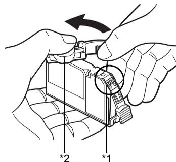
\*1 Do not touch the electrical contacts on the ink tank. Doing so can cause the machine to malfunction or become unable to print.
