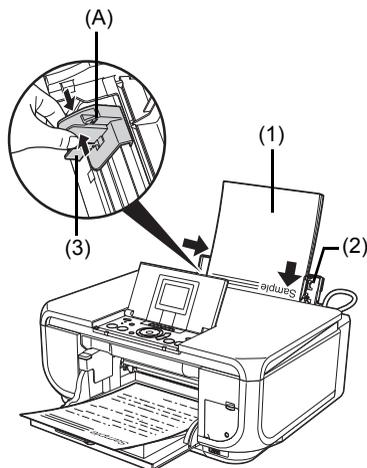
Do not load higher than the Load Limit Mark (A).
