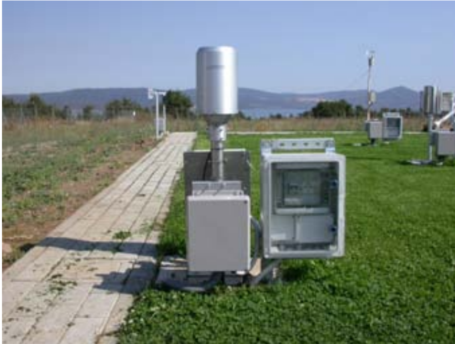
Figure A.10: Gauge 15188, LAMBRECHT, GERMANY as installed @RESMA Test Field in Vigna di Valle (Italy)
