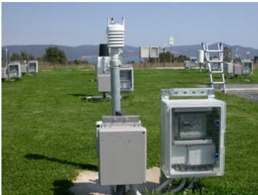
Figure A.22: Gauge WXT510, VAISALA, FINLAND as installed @RESMA Test Field in Vigna di Valle (Italy)
