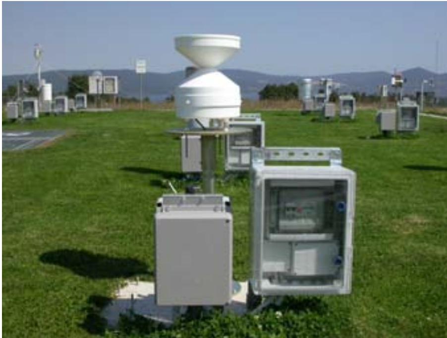
Figure A.12: Gauge ARG100, Environmental Measurements Limited, BRAZIL/UK as installed @RESMA Test Field in Vigna di Valle (Italy)
