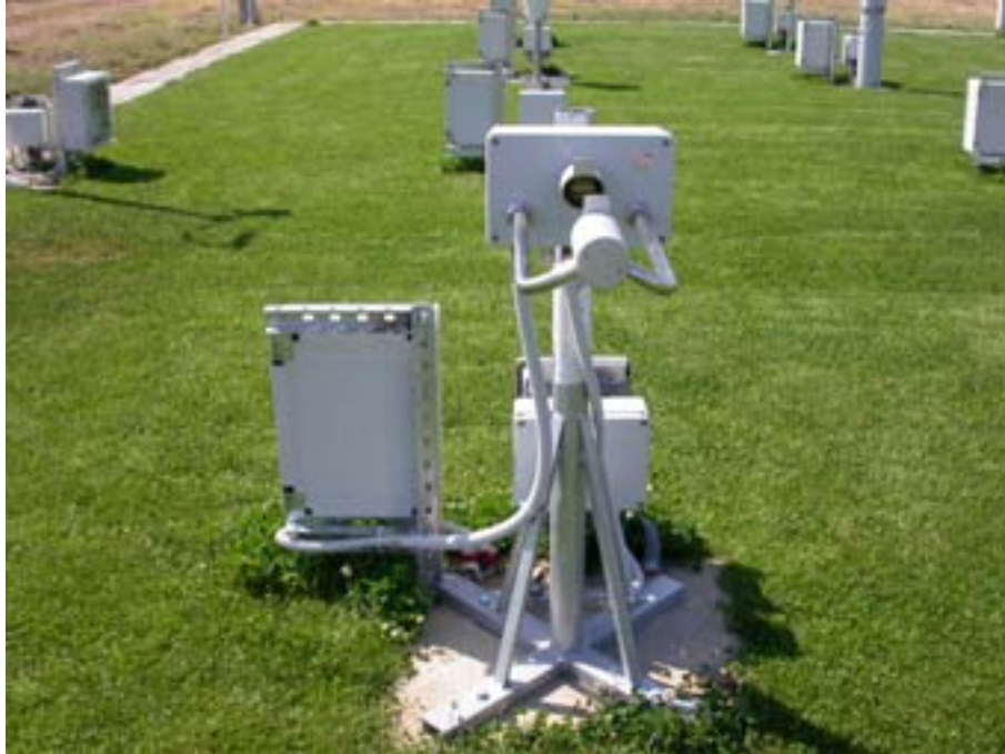
Figure A.21: Gauge LPM, THIES, GERMANY as installed @RESMA Test Field in Vigna di Valle (Italy)
