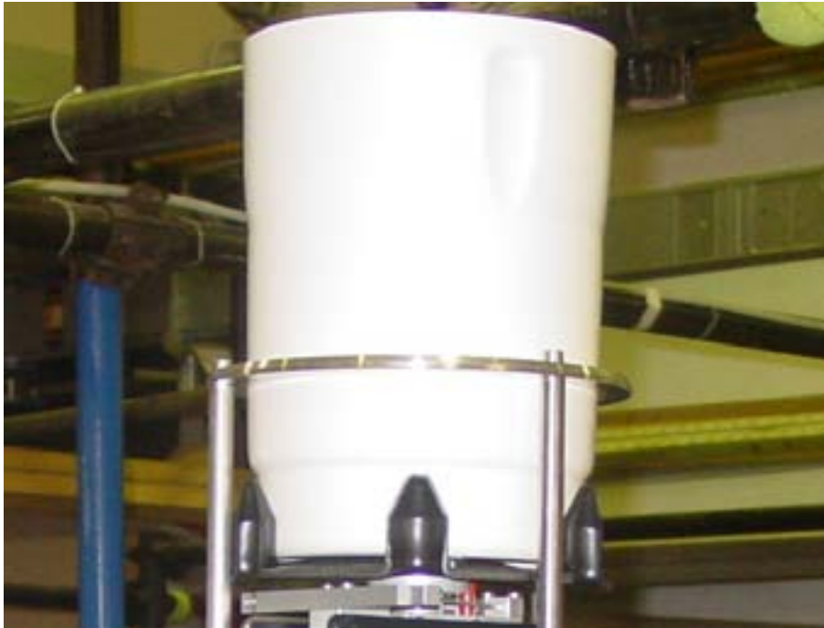
Figure A.15: PLUVIO, OTT, GERMANY as installed @RESMA Test Field in Vigna di Valle (Italy)
