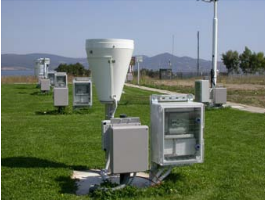
Figure A.3: Gauge R01 3070, PRECIS-MECANIQUE, FRANCE as installed @RESMA Test Field in Vigna di Valle (Italy)
