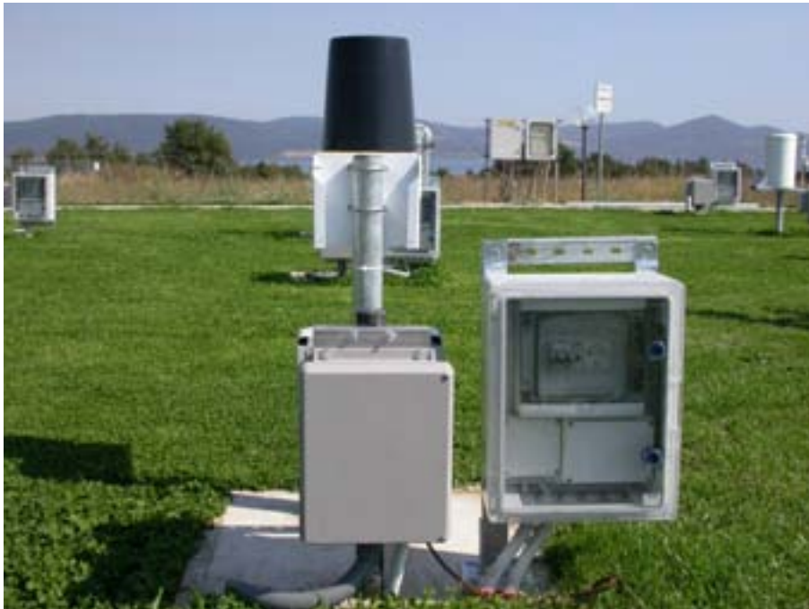
Figure A.9: Gauge RAIN COLLECTOR II (7852), DAVIS, USA as installed @RESMA Test Field in Vigna di Valle (Italy)
