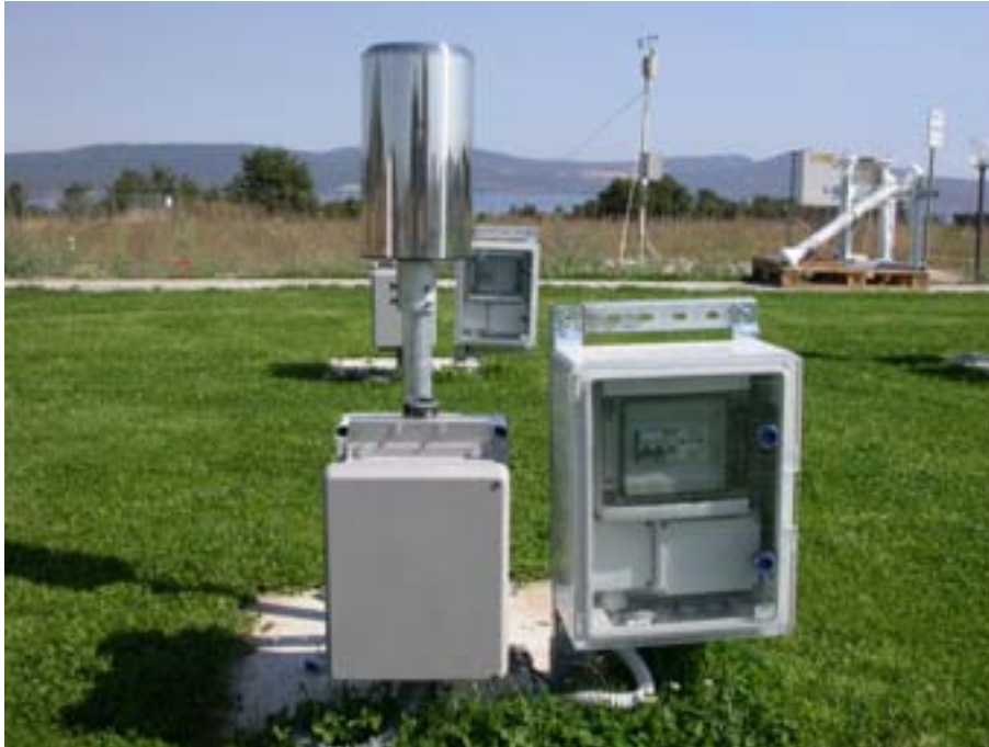
Figure A.4: Gauge PT 5.4032.35.008, THIES, GERMANY as installed @RESMA Test Field in Vigna di Valle (Italy)
