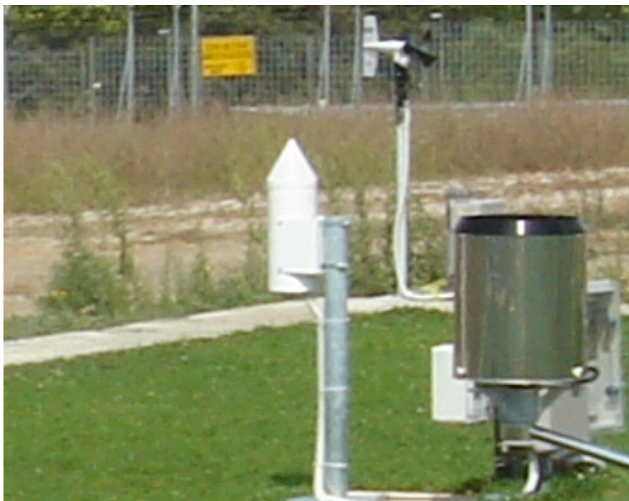
Figure A.25: Gauge DROP, PVK-ATTEX, RUSSIAN FEDERATION as installed @RESMA Test Field in Vigna di Valle (Italy)
