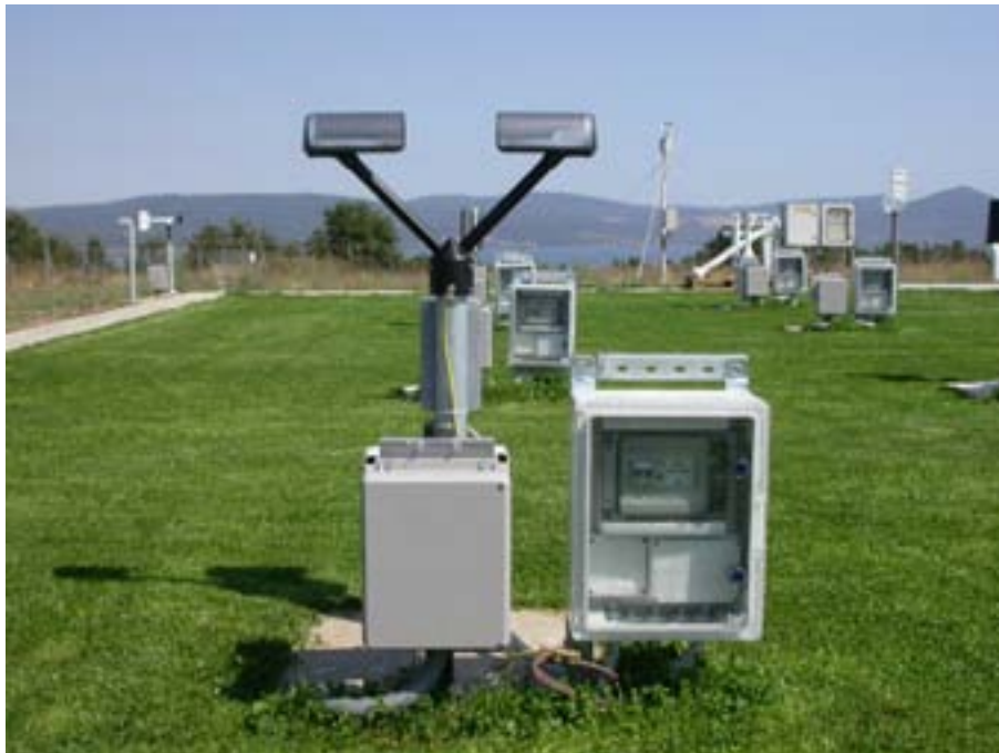
Figure A.20: Gauge PARSIVEL, OTT, GERMANY as installed @RESMA Test Field in Vigna di Valle (Italy)
