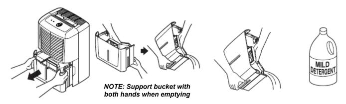
NOTE: When the bucket is full or removed from the machine, the compressor will turn off, but the fan will continue to run for a few minutes. This is completely normal. The dehumidifier will not be removing moisture from the air at this time.
