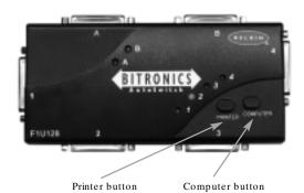
To use File Transfer mode, press the PRINTER button until the LED on the computer port turns green. When the LED turns green, the port is ready for file transfer mode. For file transfer mode to be successful for both PCs, both computer ports must be set to file transfer mode – which is evident when the LEDs next to 1 and 2 are green. For more information on File Transfer, please see page 25.
