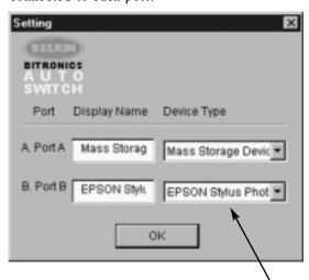
Device Type gives you a pull-down menu showing the types of printers installed on your computer and other possible parallel device types as well.
