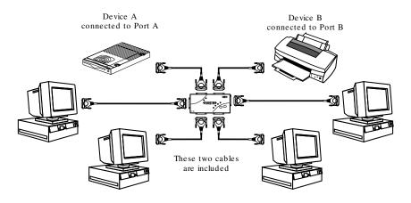
Connect the power adapter to the power jack on the side of the switch, and plug it into an outlet. The example shown has a Zip® Drive connected to Port A and an InkJet printer on Port B of the switch.
