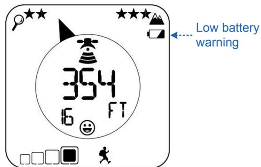
**Figure 19:** The low battery warning symbol.
