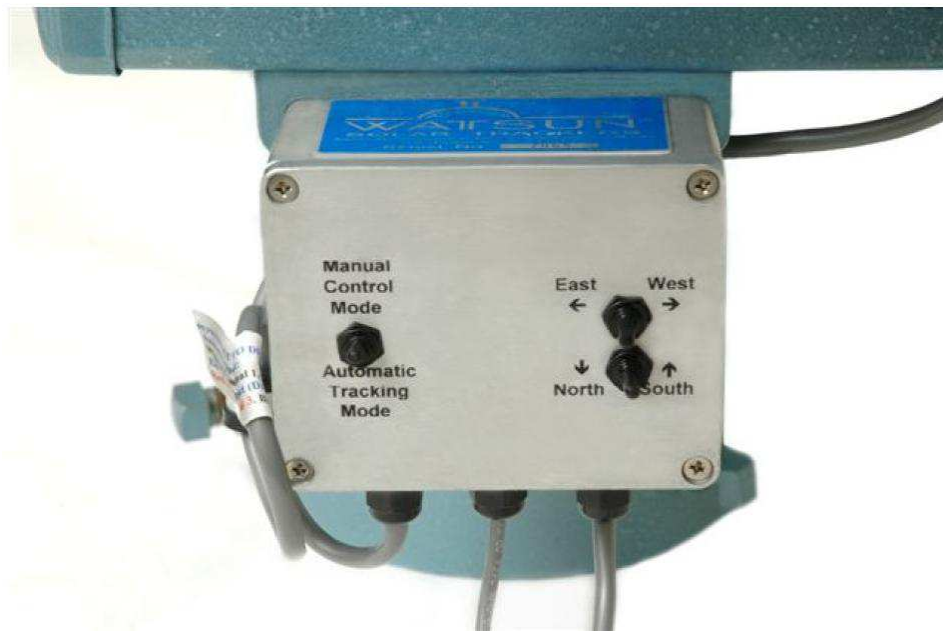
Figure 11: Dual-axis tracker Manual Controls
