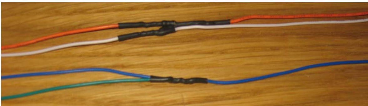
Figure B5: Position and heat the shrink tubing to protect the joints.
