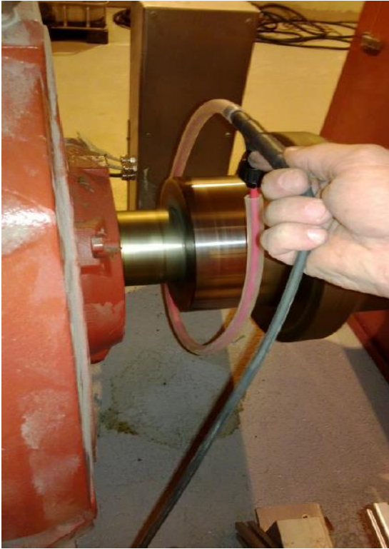
Figure 25. Measuring the shaft grounding current from the axis. A Rogowski probe is held around the rotating axis.
