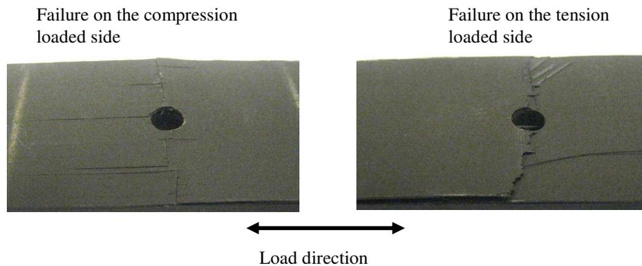
Fig. 3. Compressive (left) and tensile failure of a 8 mm thick specimen with a 6 mm hole.
