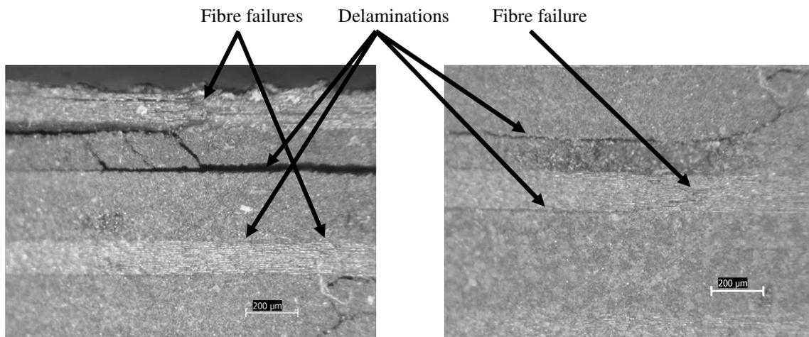
Fig. 7. Fibre failure, matrix cracks and delaminations in the tensile loaded side of the specimen. Left layer 1-7 and right layer 6-13 from the surface.
