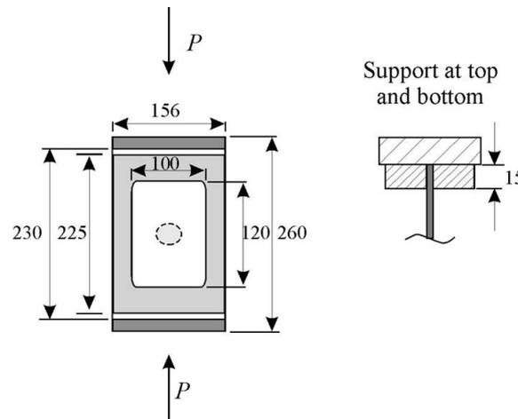
Fig. 2. Antibuckling device used during compression tests of the 156 mm wide specimens.
