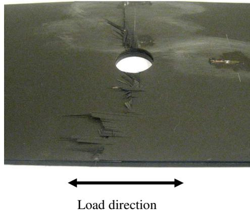
Fig. 4. Tensile failure of a 4 mm thick specimen with 25 mm hole.
