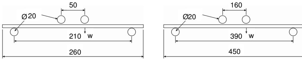
Fig. 1. Bending tests of laminate with 6 mm hole (left) and 25 mm hole (right) respectively.
