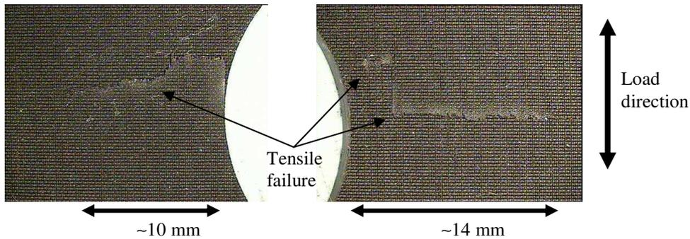
Fig. 5. Initiation of tensile failure in a 4 mm thick specimen with 25 mm hole.
