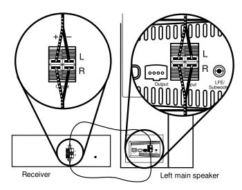
Press down the terminal tab on the bottom of the left main speaker to insert the appropriate wire (Figure 5).
