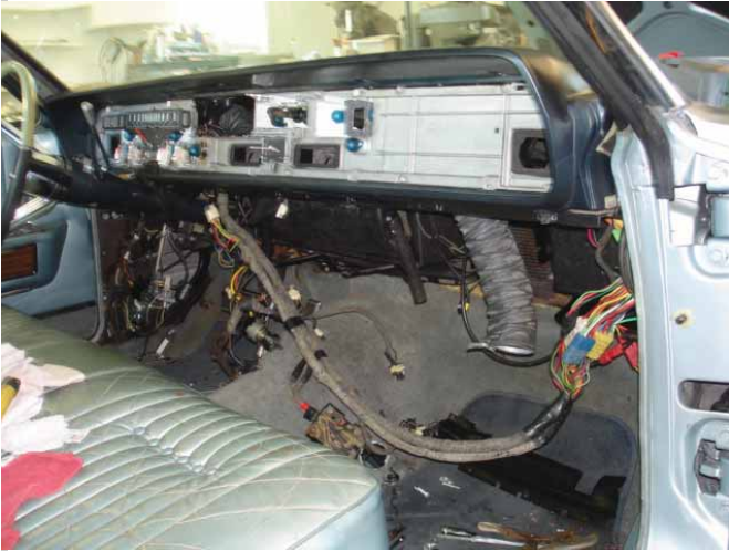
New Wire Loom Installed Before Dressing Into Place
