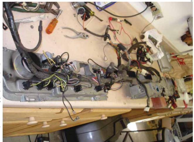
Dash Panel on Bench Receiving New Wire Loom
