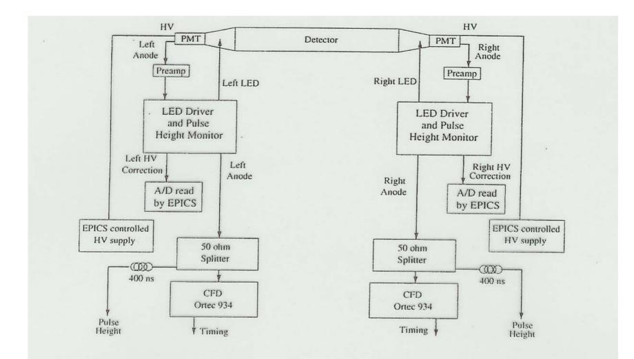
Figure 3.4: This is a schematic of the electronics used to produce the timing and pulse height signals for the 44 neutron detectors in NPOL. All electronics were installed in the NPOL detector enclosure under the detector platform.
