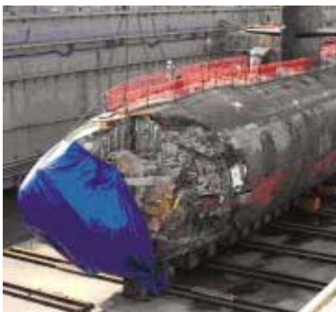
Photo showing the damage sustained to the USS SAN FRANCISCO (SSN 711). USS SAN FRANCISCO is the 24 th submarine in the LOS ANGELES class and the sixth ship of that class built by Newport News Shipbuilding in Newport News, VA. She was commissioned on 24 April 1981.
