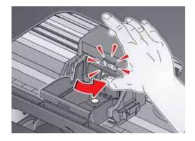
10. Insert the black ink cartridge into the printhead.
