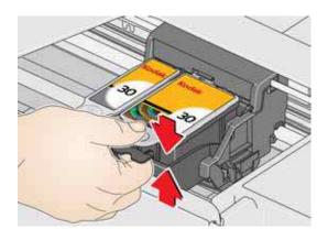
4. Lift the ink cartridge out of the printhead.
