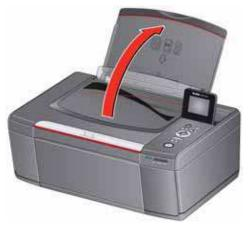
2. Open the paper output tray, then pull out the extender until it is fully extended.
