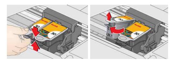
4. Unlatch the used printhead by lifting the button in the center of the carriage.
