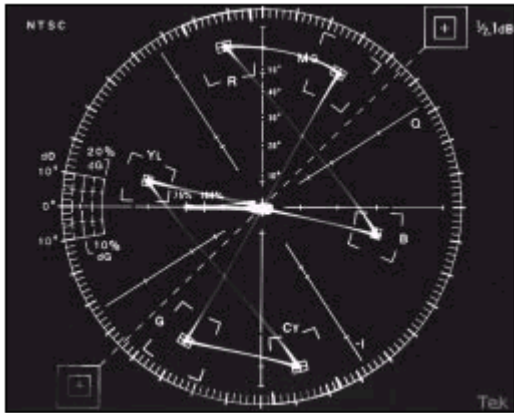
Vectorscope Display of SMPTE Bars
