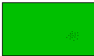
Missing (stuck) Pixels
