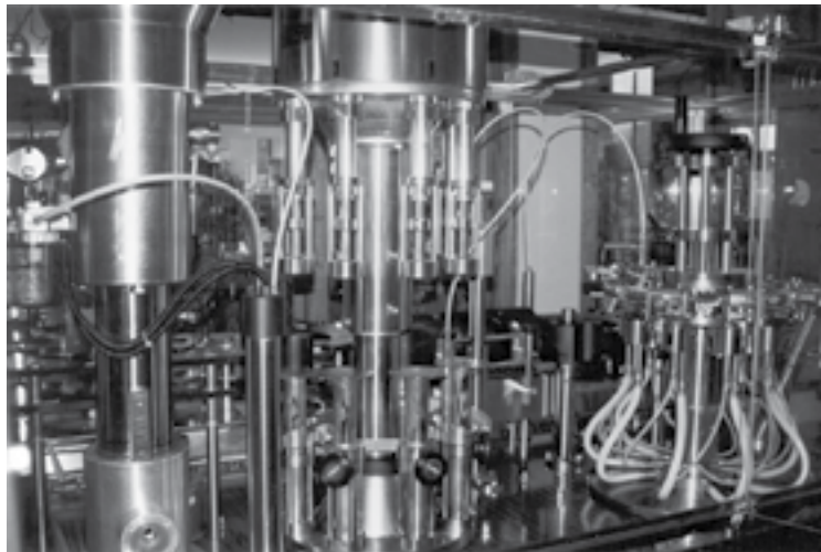
Equipment in a commercial food-processing facility is generally made of stainless steel, which allows for adequate cleaning and sanitizing.
