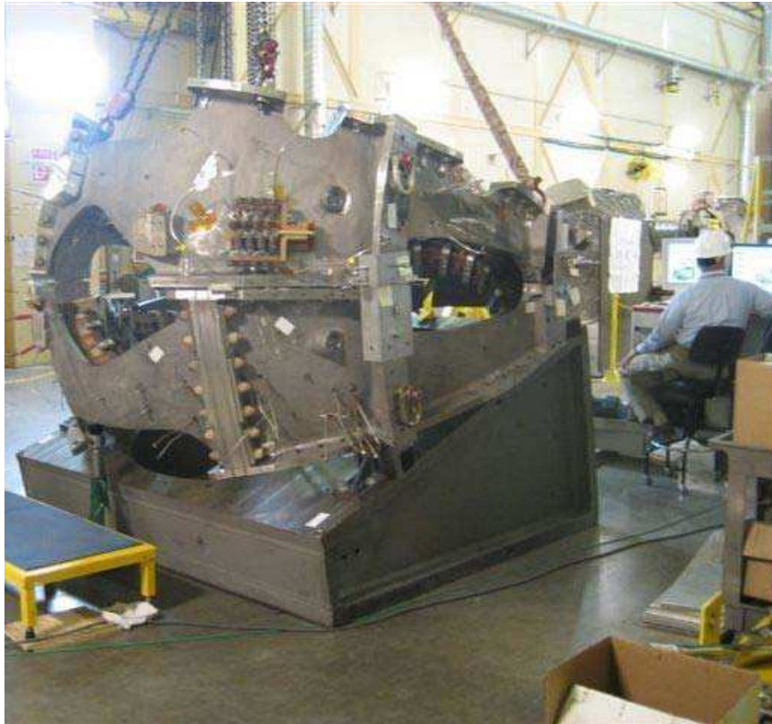
Figure 4 Mating “B” Coil into Position
