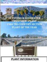
The El Estero WWTP is an 11 million gallons per day Secondary Treatment Facility equipped with a 4.3 million gallons per day Water Reclamation Treatment Facility. At present flow rate, the secondary treatment system is operating at approximately 70% of its capacity, while the recycled system is operating at 42% of its capacity. The El Estero facilities are designed to meet the needs of the City well into the twenty-first century.
