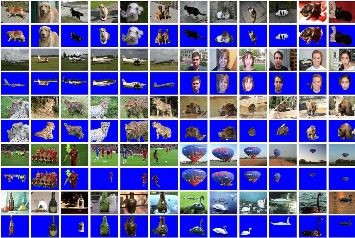
Fig. 5. The segmentation results of the proposed method. From top to bottom: the rows 1, 3, 5, 7 and 9 show the original images. The rows 2, 4, 6, 8 and 10 display the segmentation results.
