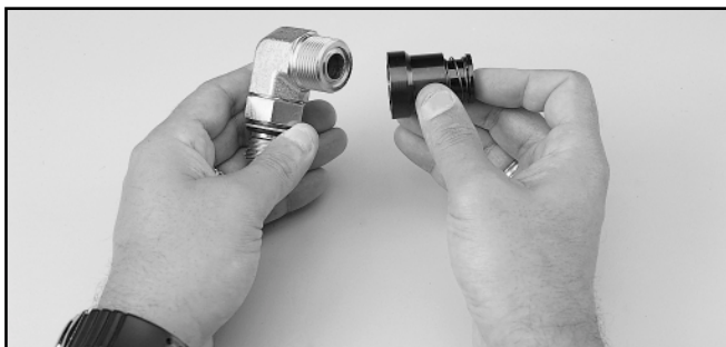
Figure I10 — O-Ring Installation Using CORG Assembly Tool
