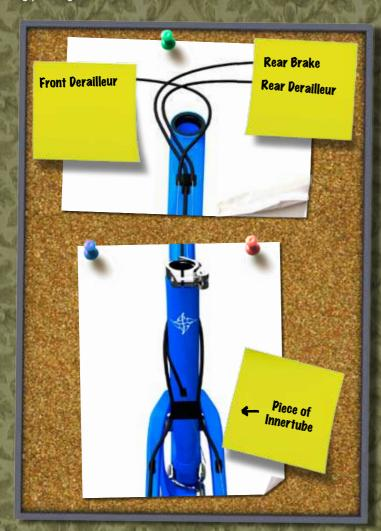
We recommend you use a piece innertube about 3 cm long, feeding the rear brake and derailleur cables through it just behind the seat tube as shown. Zip Ties work well too.
