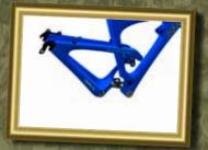
Notice that the two upper links are being pulled across the seat tube where the front derailleur mounts.
