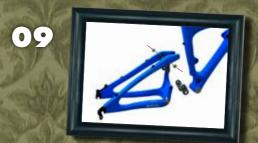
Remove the remaining screws in the upper links of the swingarm with a 5 mm Allen wrench as well.
