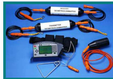
OhmMapper portable capacitively coupled resistivity imaging system for levee inspection
