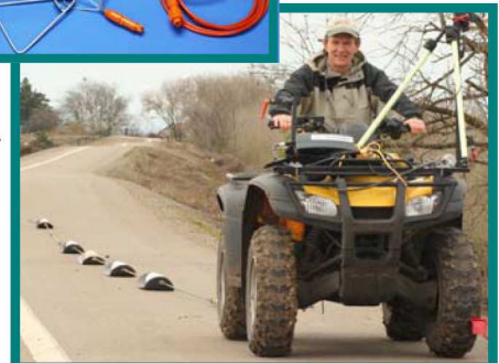
OhmMapper resistivity system can be vehicle towed and operate over concrete and asphalt
