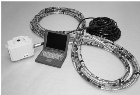
The DHA-6500 connected to a Geometrics GEODE seismograph
