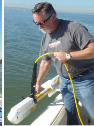
Deploying Geometrics G-882 ultra-sensitive marine magnetometer
