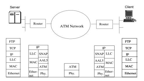
The following figure shows a network that supports video-on-demand using ADSL. The protocol stack is also presented.
