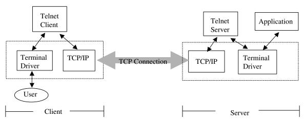
The client operating system provides the terminal driver and the TCP/IP protocol. The user invokes and input to the Telnet client via the terminal driver. The client Telnet then requests a TCP connection to the server.
