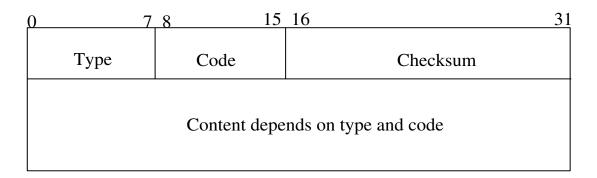
Type field is used to identify the ICMP message. There are 15 different types. Each type may have different codes to provide further information. The 16-bit checksum covers the entire ICMP message.
