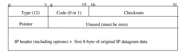
The code indicates the problem. The pointer field identifies the octet in the datagram's header that causes problems.
