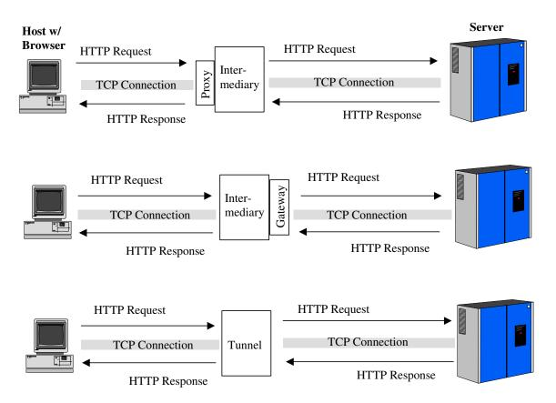
The proxy can be a firewall of a network, and the client is part of the network. The proxy acts as a server in interacting with a client, and as a client in interacting with a server. The proxy can also serve as an intermediary if the client and the server are running different version of HTTP. In this case, the proxy implements both versions and performs the mapping.
