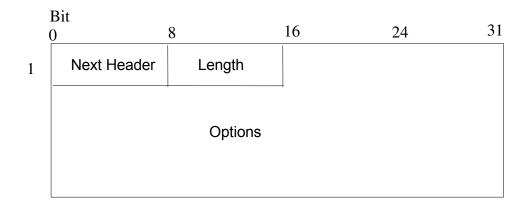
Where length is the length of the header. Each option consists of three fields: Type (8 bits), Length (8 bits) and Value (variable length).
