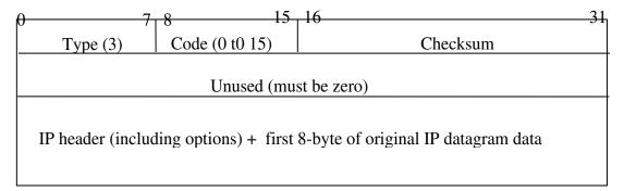
The code field describes the problem. ICMP message includes a short prefix of the IP datagram that can not be delivered. This information will let the originating host know exactly which datagram causes problem. Note that the first 8-byte of the IP datagram data could include the
