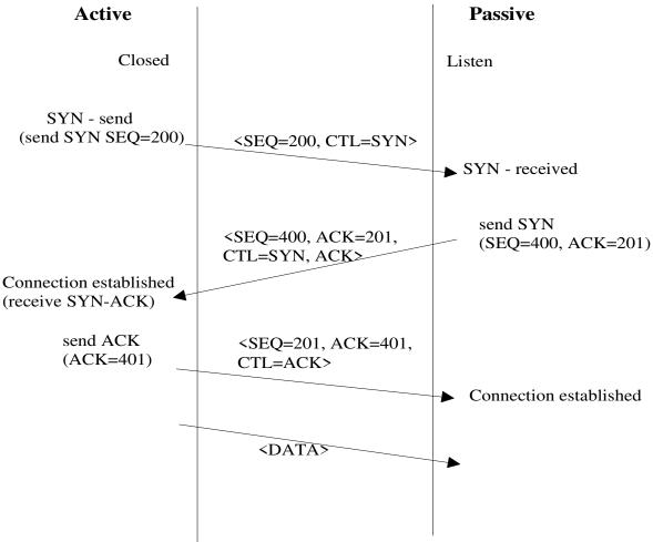
Once the connection is established, the two computers start to send and receive data packets.
