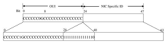
Note that the C bits in the OUI portion of the MAC address are used to identify the company. The 6<sup>th</sup> bit in the first byte of the MAC address, which is used to indicate whether the address has global scope, is changed from to 0 to 1.
