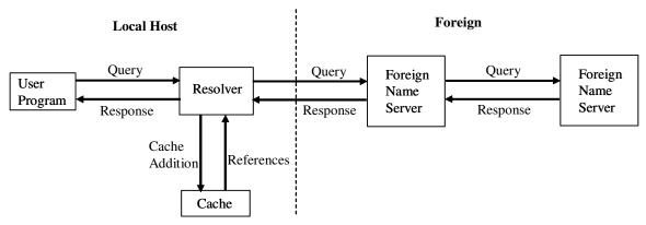
Domain Name System uses the service of UDP or TCP, with the port number of 53. The format of the DNS messages is as following:
