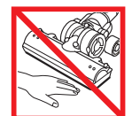
Do not put hands near the brush bar when the vacuum cleaner is in use.
