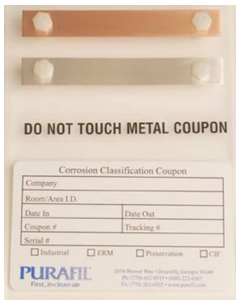
Figure 1: Picture of an Unexposed Corrosion Classification Coupon
