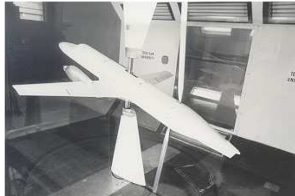
Figure 16. Two strut mount with image system.
