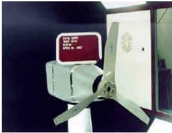
Figure 43. Propeller test with single strut mount.
