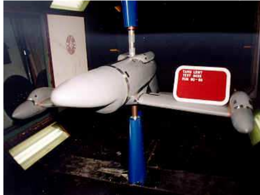
Figure 18. Image system with a single strut
