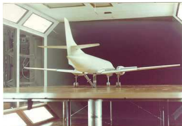
Figure 27. Ground plane with single strut mount.
