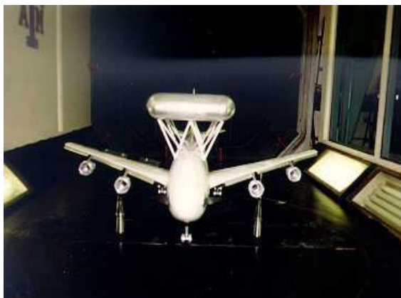
Figure 26. Variable height three strut mount.
