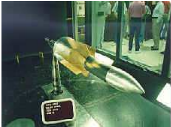
Figure 22. Missile with the small sting mount.
