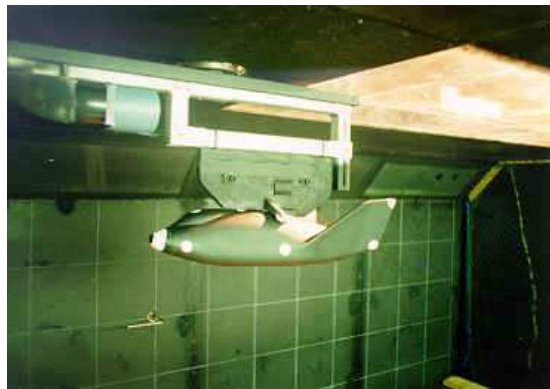
Figure 36. NASA X-38 drop model set-up.
