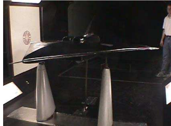
Figure 12. Three strut mount.
