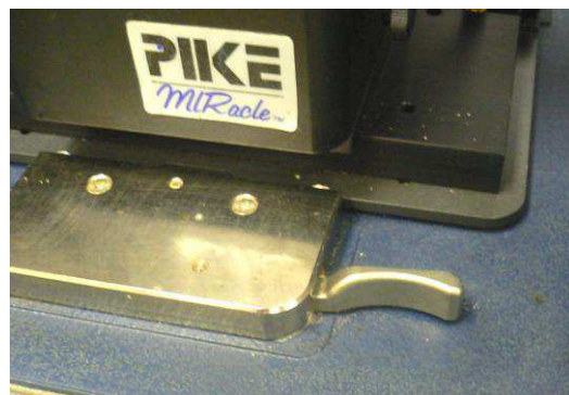
Figure 8. Cell base plate unlocking lever.
