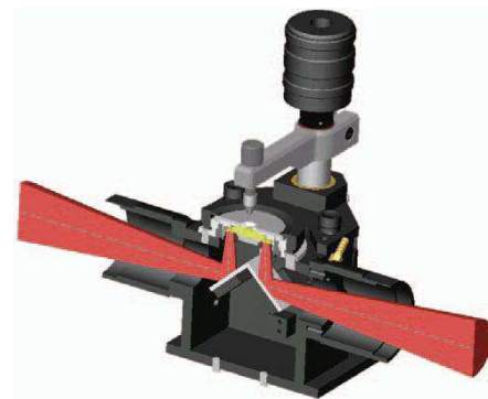
Figure 3. IR beam path for Pike ATR cell.
