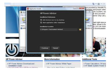
The next screen will allow the user to determine whether a shortcut is added to the desktop. This screen also allows for the automatic start of the application after installation. Finally, the user can define a location for the tool – the default location is C:\Program Files\Hewlett-Packard. Once the preferred selections are made, left mouse click on the "Continue" button.
