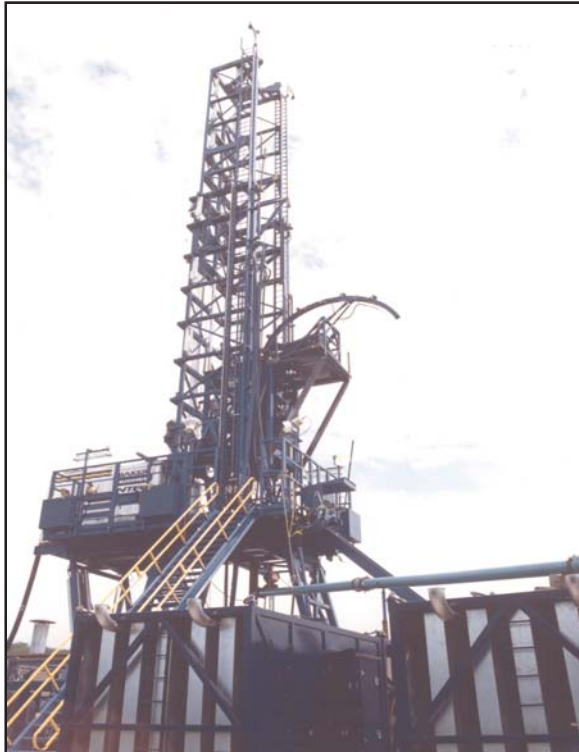
Figure 16: CT Drilling Unit Mast and Substructure for CT Sizes through 5 1/2 in.
