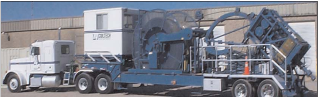
Figure 8: CT Unit Rigged Down for Highway Transport
