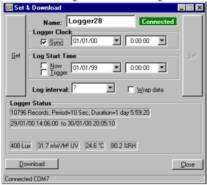
If "Auto Download" was checked then any new data is downloaded automatically. Otherwise, if required, click on the Download button to start transmission. The infrared link is closed after all data has been sent.
