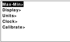
The first menu item "Max-Min" is highlighted, different menu items can be highlighted using the  $\emptyset$  and  $\times$  buttons. The wanted action is done by highlighting the appropriate menu item and pressing the Set button. To abort without doing anything press the X button. In some cases a further sub-menu is displayed with more choices.
