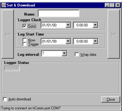
If "Auto Download" is checked then any new data is downloaded as soon as contact is made with the logger.
