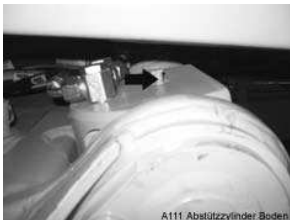
Ground support cylinder
