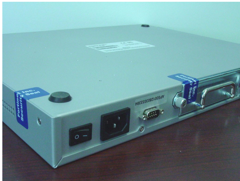
Figure 6: FortiGate-300, 400 and 500 tamper seal placement
