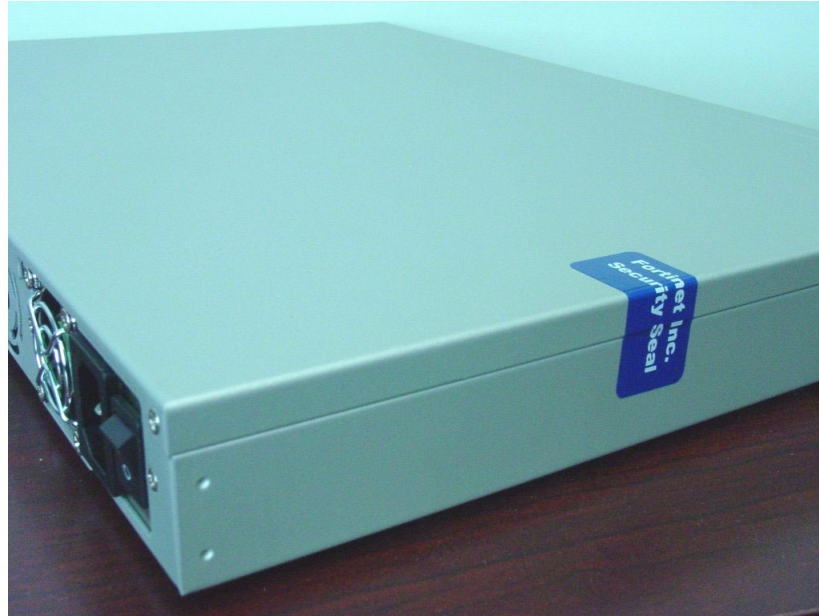
Figure 7: FortiGate-800 tamper seal placement
