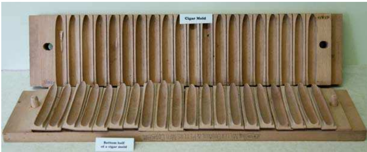
A cigar mold showing top and bottom halves.
