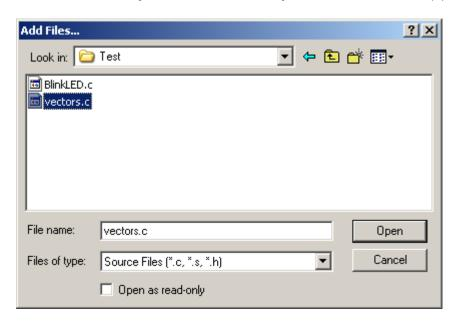
Note that ICC12 has changed to include **vectors.c** It is important to note that the **vectors.c** was written for the 68HC912B32 and 812A4 MCUs. One should edit the file to include other ISR addresses for the 9S12C32. This example uses the file as is.
