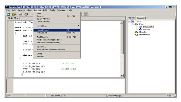
Note the bottom window pane will show messages to display how the build progressed. Any errors, if any, are shown in this window. The build was without error so we can progress to erasing and programming the 9S12C32.
