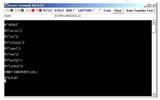
Note the "Connect" message that lists the Bluetooth address of the connected device, the profile (UUID) in use and the direction of the connection.
