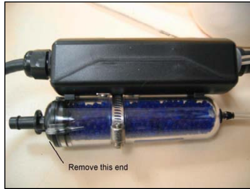
Figure 5. Flow meter desiccant
