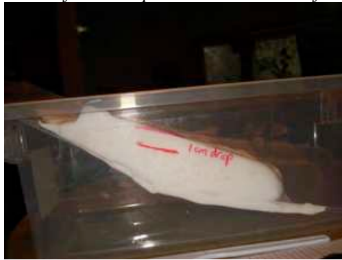
Image 12) Mark up surface and 1 cm drop Image 13) Time goo as it drops 1 cm Repeat 2 other times, or pool class results for an average.
