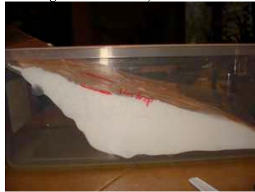
Image 12) Mark up surface and 1 cm drop Image 13) Time goo as it drops 1 cm Repeat 2 other times, or pool class results for an average.
