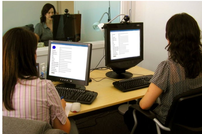
Figure 8. Our eye tracking lab setup. The participant (to the right) is sitting in front of the Tobii eye tracker, while the session moderator (to the left) is controlling the eye tracking software and administering the tasks. The moderator is also able to see the participant's eye movements in real time (indicated by a blue dot moving across the screen).
