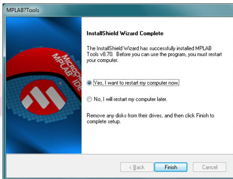
Click the “Finish” button and restart you computer to finish install the MPLAB IDE.
