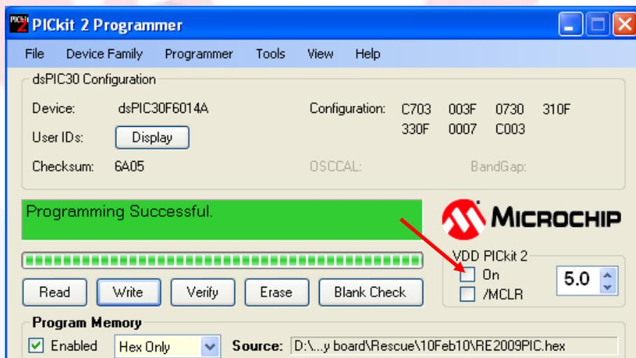
Step 5: You can turn on the controller board by clicking on the “On” button to test the controller board. However, the voltage provided by the PC is not strong enough to power the motor.
