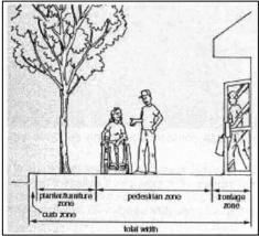
opening into the sidewalk corridor, two feet of width should be provided.
