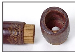
There were separate housings at either end for the objective and the eyepiece
