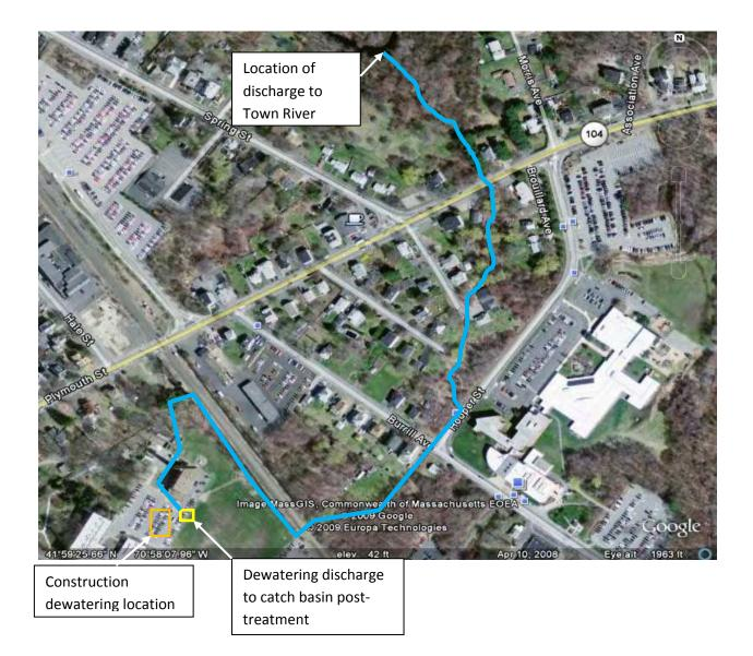
Plan Showing Route of Dewatering Discharge to Catch Basin (post-treatment) and Route to Receiving Water (Town River)
