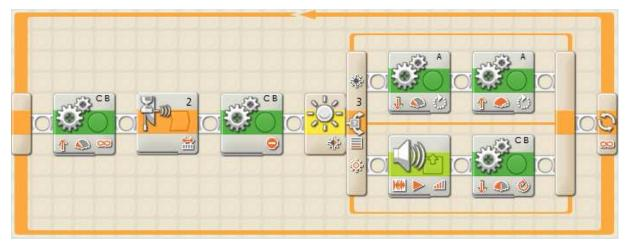
The above program makes the NXT move forward until it is close enough to a ball and then it hits the ball only if it is of a particular colour.
